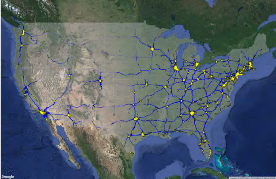
Figure 16. U.S. Interstate Highway corridors. Line thickness is proportional to HPMS average daily traffic.
