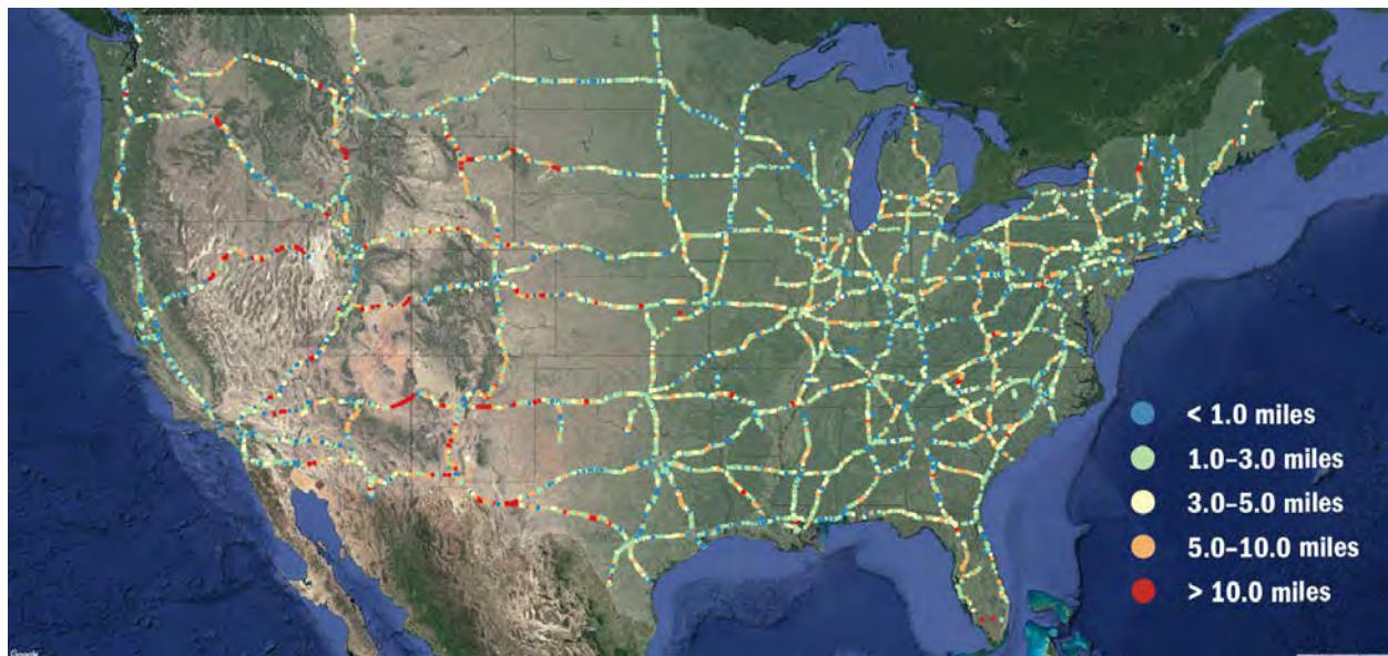
Figure 31. Highway exits color-coded by distance to the nearest electrical substation. (Satellite imagery credit: © 2017 Google, Map Data © 2017 Tele Atlas)
