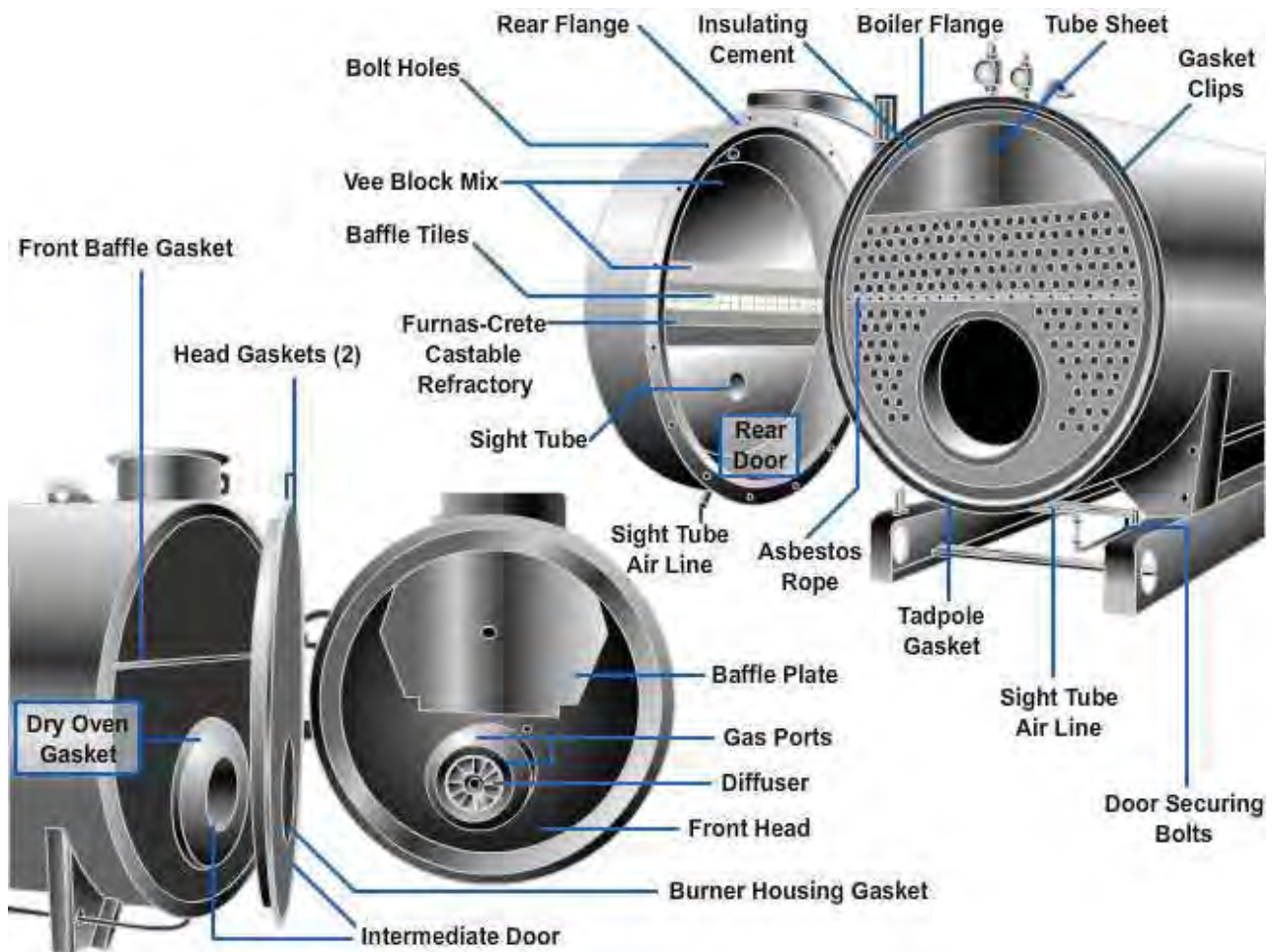
Figure 54 - Front and rear doors open on a gas-fired boiler.
