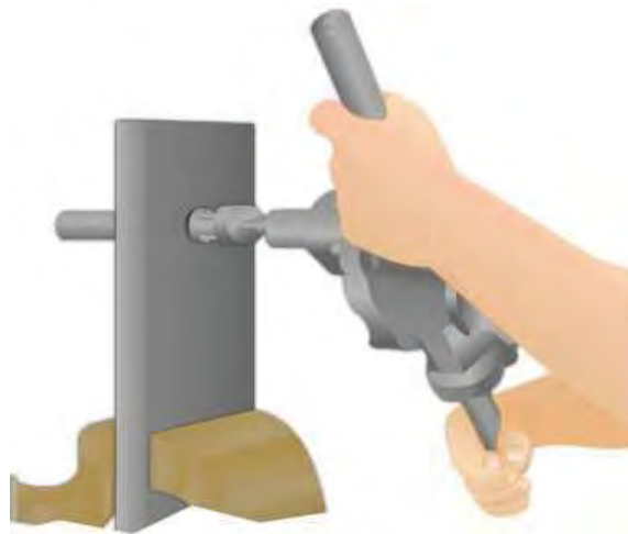
Figure 46 -Expanding a tube.
