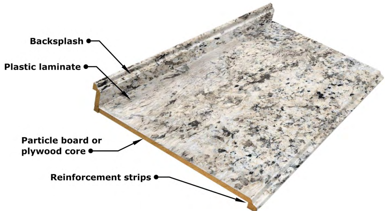
Figure 2.24 Typical countertop with plastic laminate cover
