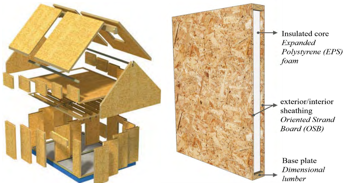
Figure 3.9 Left: Exploded Axonometric of a SIPs Building. Right: Traditional SIP panel fabricated from OSB and expanded polystyrene (EPS) insulation. (Source: Homebuilding & Renovation)
