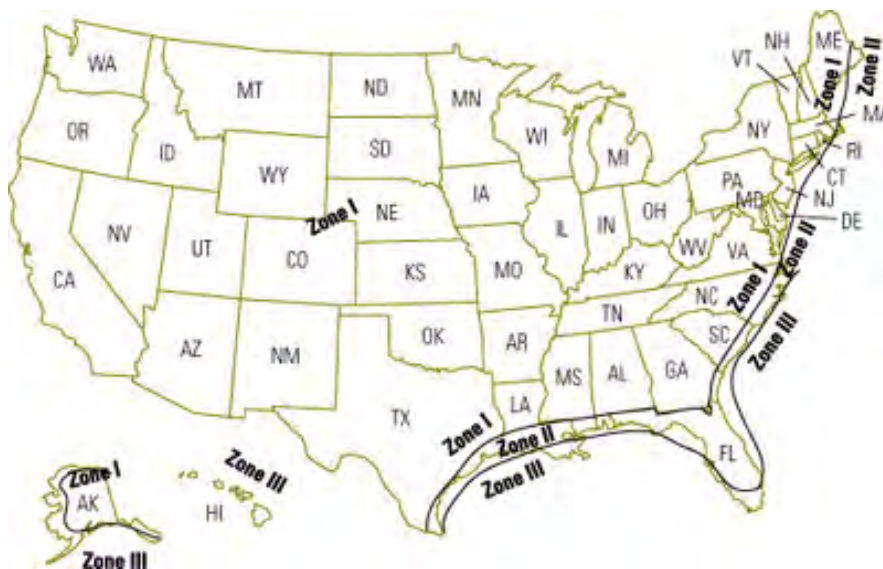
Figure 1.6 There are three Wind Zones in the HUD Code, with Wind Zone III designating the highest wind velocities. The higher the Wind Zone, the more stringent are the requirements for connecting the home and its components together and to the ground.
