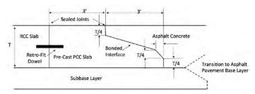
**Figure 11.** Transition of RCC/AC pavement interface [10].
