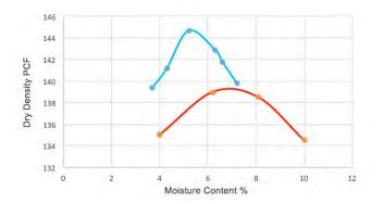
Figure 2. RCC mixture moisture sensitivity.
