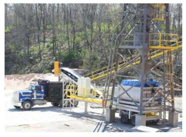
Figure 6. Twin shaft horizontal mixer—batch type.
