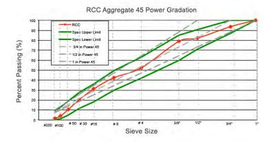
Figure 1. Example RCC concrete gradation.
