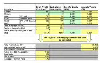
Figure 4. Typical RCC mixture proportions.
