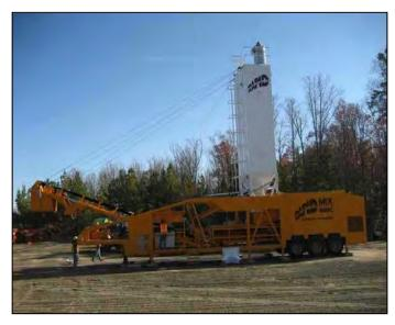
Figure 7. Twin shaft horizontal mixer—continuous type.
