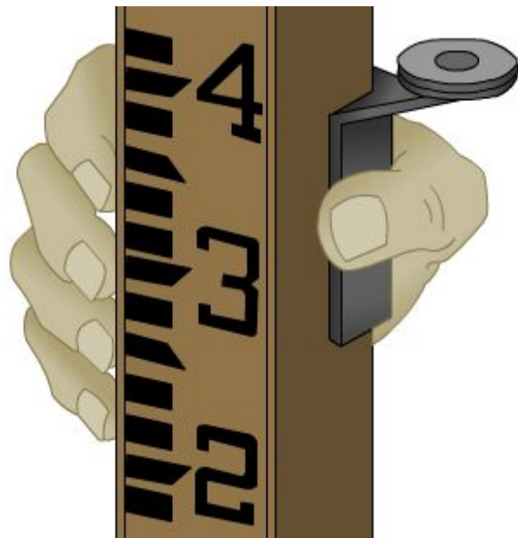
Figure 25 – Bull's eye rod level.
