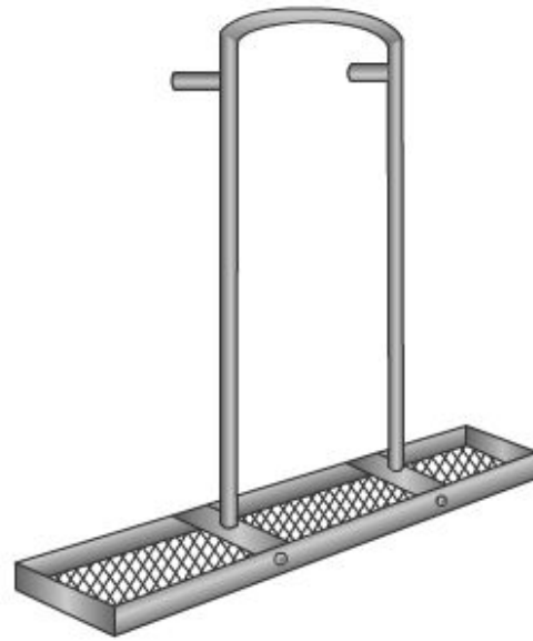
Figure 68 – Hand tamp (Jitterbug)
