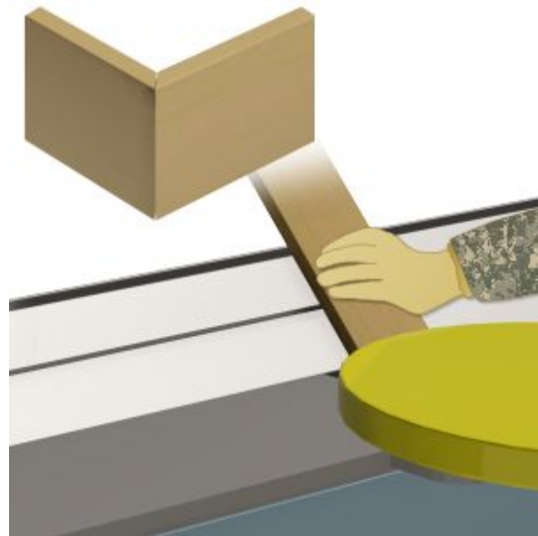
Figure 24 – Beveling on a jointer for a mitered edge joint.
