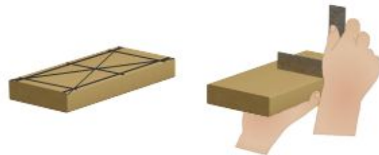
Figure 12 – Working the face.
