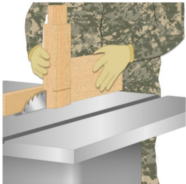
Figure 34 – Making tenon cheek cut on a table saw using a push board.
