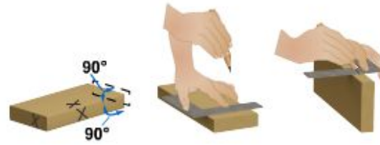
Figure 15 – Working the second end.
