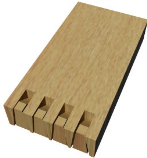
Figure 41 – Chiseling out waste in a through multiple dovetail joint.
