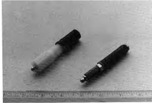
Figure 16-3 Typical Injection Ports for Chemical Grout
