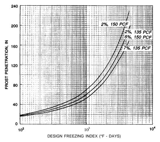
Figure 18-3. Frost Penetration Beneath Pavements. (Sheet 1 of 3)
