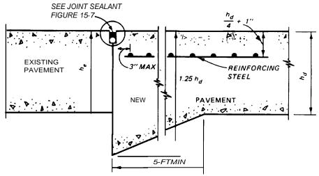
NOTE: THIS TYPE JOINT SHOULD BE USED ONLY WHEN EXISTING PAVEMENT IS TO BE REPLACED IN A SHORT PERIOD OF TIME, SINCE WITHOUT LOAD TRANSFER, IT WILL DETERIORATE QUICKLY.
