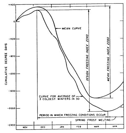
Figure 18-1. Determination of Freezing Index.
