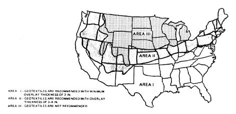
Figure 14-2. Location Guide for the Use of Geotextiles in Retarding Reflective Cracking.
