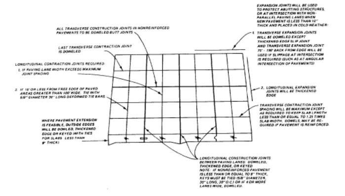
Figure 15-2. Joint Layout for Vehicular Parking Areas.
