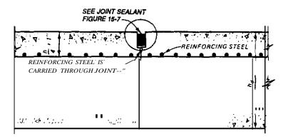
NOTE: SAW CUT Will NOT EXTEND BELOW STEEL REINFORCING
