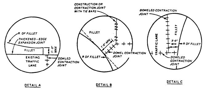
Figure 13-1. Typical Layout of Joints at Intersection. (Sheet 2 of 2)
