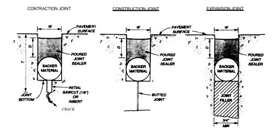
W +WIDTH OF SEALANT RESERVOIR (SEE TABLE) D + DEPTH OF SEALANT (1.0 TO 1.5  $\rm X$  W) T + DEPTH OF INITIAL SAWCUT OR INSERT TYPE JOINT FORMER ICONTRACTION JOINT)
