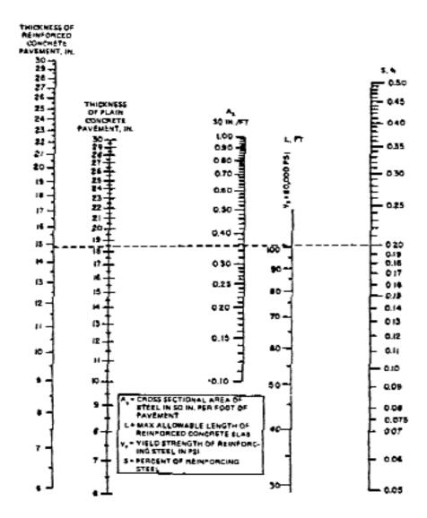
Figure 13-2. Reinforced Rigid Pavement Design
