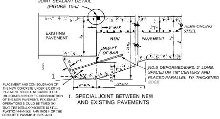
Figure 16-2. Construction Joints for Reinforced Concrete Pavements. (Sheet 3 of 4J
