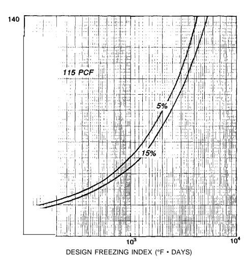
Figure 18-3. Frost Penetration Beneath Pavem€nts. (Sheet 2 of 3)
