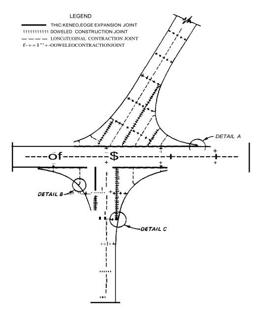
Figure 13-6. Typical Layout of Joints at the Intersection of Reinforced Rigid Pavement. (Sheet 1 of 2J
