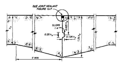
A TOLERANCE OF ± 1/16" MAY BE ALLOWED FOR KEY DIMENSIONS AND LOCATION
