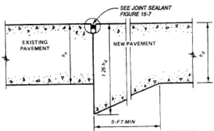
NOTE: THIS TYPE JOINT SHOULD BE USED ONLY WHEN EXISTING PAVEMENT IS TO BE REPLACED IN A SHORT PERIOD OF TIME, SINCE WITHOUT LOAD TRANSFER IT WILL DETERIORATE QUICKLY!
