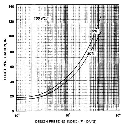
Figure 18-3. Frost Penetration Beneath Pavements. (Sheet 3 of 3)
