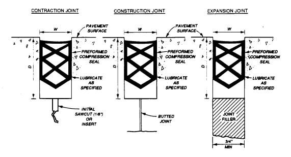
DEPTH & WIDTH: AS RECOMMENDED BY MANUFACTURER PER TYPE OF SEAL BEING USED, (DEPTH NOT LESS THAN 1.5 INCHES)
