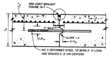
A TOLERANCE OF ± 1/16" MAY BE ALLOWED FOR KEY DIMENSIONS AND LOCATION A VERTICAL TOLERANCE OF ± 1/4" IS ALLOWED FOR PLACEMENT OF TIE BAR
