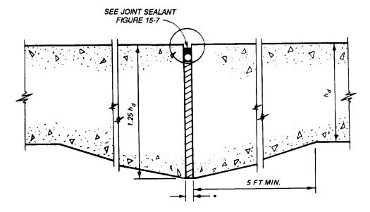
THE BOND-BREAKING MEDIUM WILL BE EITHER A HEAVY COATING OF BITUMINOUS MATERIAL NOT LESS THAN 1/16 INCH IN THICKNESS WHEN JOINTS MATCH OR A NORMAL NONEXTRUDING - TYPE EXPANSION JOINT MATERIAL 1/4 INCH IN THICKNESS WHEN JOINTS DO NOT MATCH.
