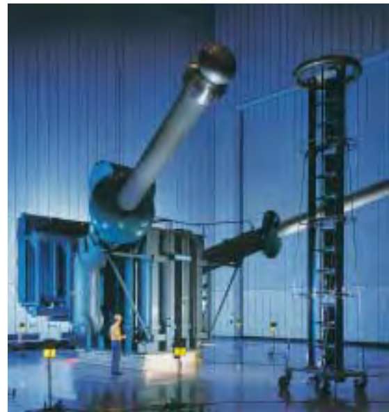
Fig. 5.3-1: Oil-insulated smoothing reactor – Three Gorges project
