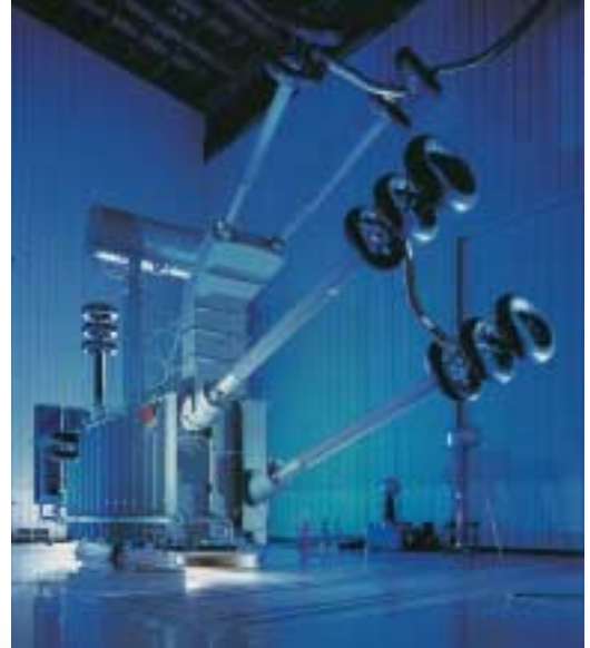
Fig. 5.2-1: Converter transformer for the Tian Guang HVDC project during type test
