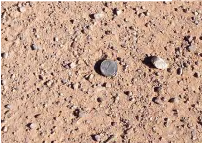
High quality surface gravel with a good blend of stone, sand and fine-sized particles on a mountain road.
