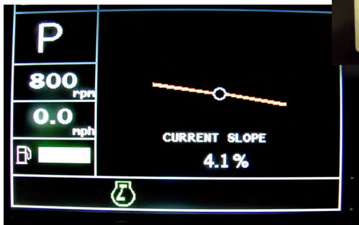
Two examples of screens in the grader cab showing electronic slope controls being used to construct at or near 4 percent crown, or cross-slope, on the road surface.
