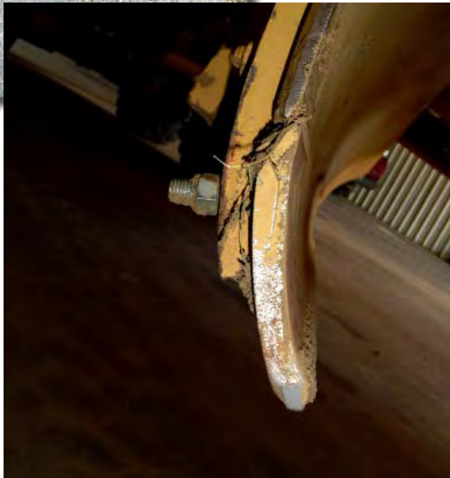
Example of carbide-insert in a cutting edge with hard facing on the bottom of the face to increase wear life.
