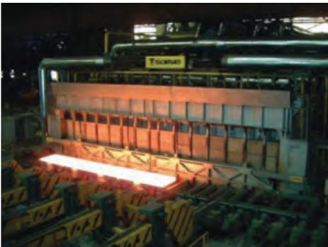
*A walking beam furnace for metal reheating.*
