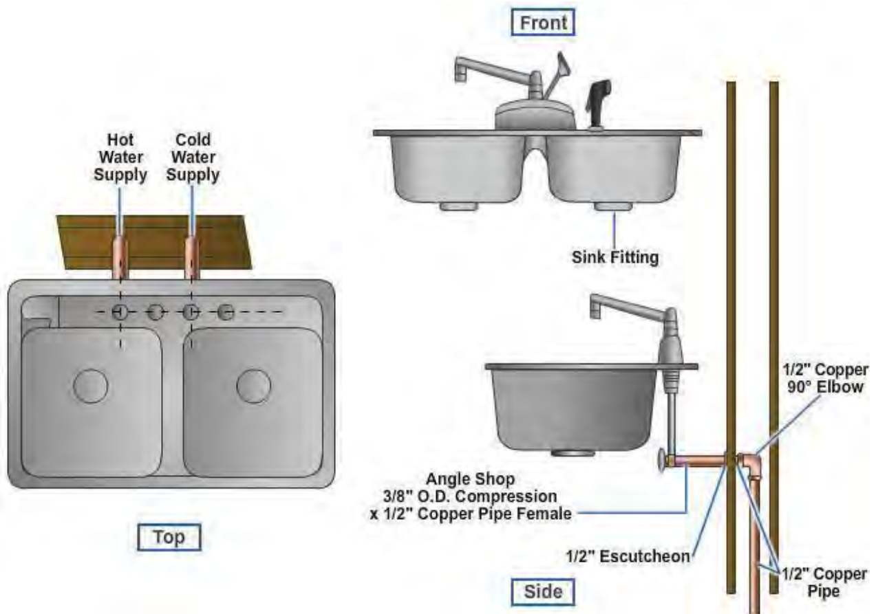
Figure 11 — Kitchen sink water supply hookup.
