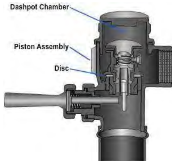
Figure 39 – Piston type trouble-flushometer valve. properly
