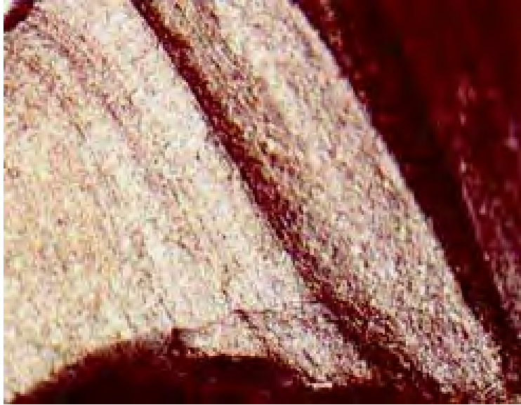
Figure 17 Characteristic Fatigue Striation Pattern 15
