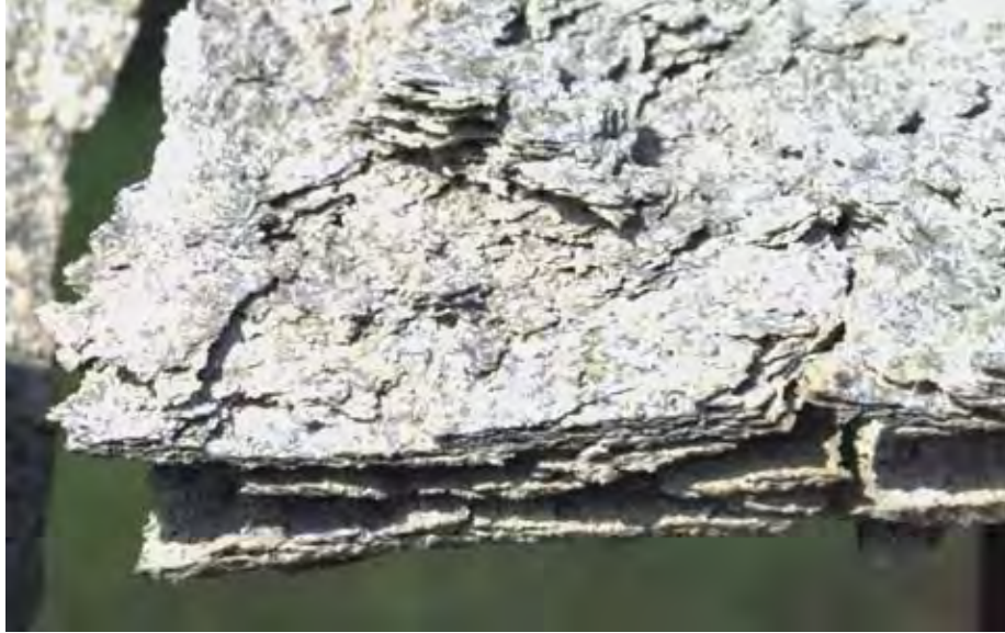
Figure 23 Exfoliation of an Aluminum Alloy in a Marine Environment 2
