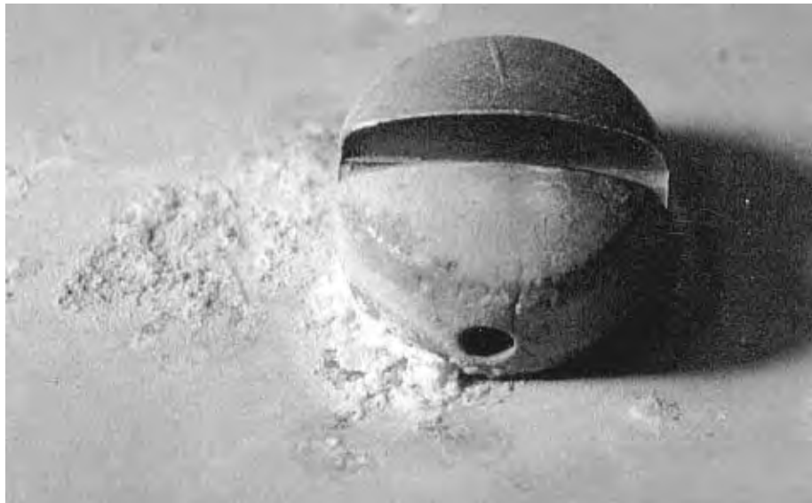
Figure 9 Galvanic Corrosion between a Stainless Steel Screw and Aluminum 2
