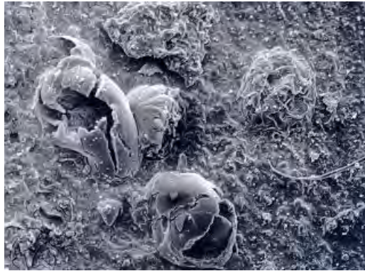
Figure 26 Tubercles as a Result of MIC (courtesy of Metallurgical Technologies, Inc.) 28
