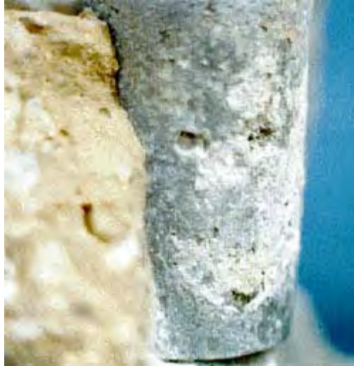
Figure 12 Pitting Corrosion of an Aluminum Railing near the Atlantic Ocean 2
