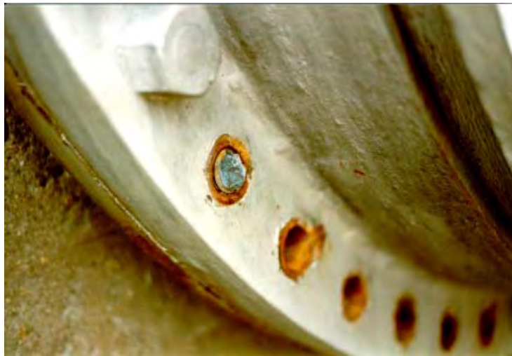
Figure 14 Dezincification of Brass Containing a High Zinc Content 13
