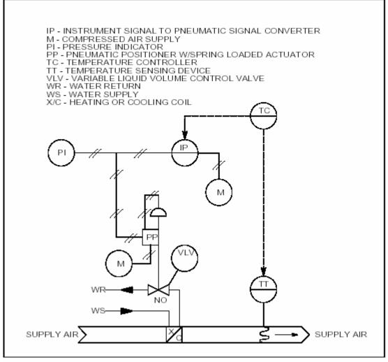
Figure 4-2. Typical HVAC control loop
