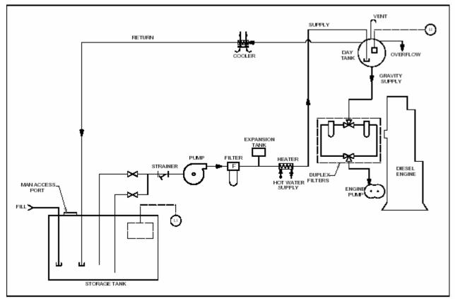
Figure 5-1 Schematic of a typical fuel system
