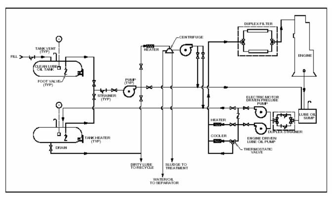
Figure 5-2 Schematic of a typical lube oil system
