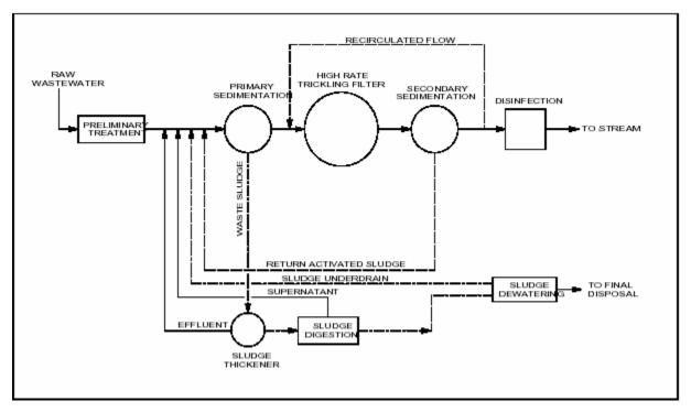
Figure 9-4 Sewage trickling Filter Process
