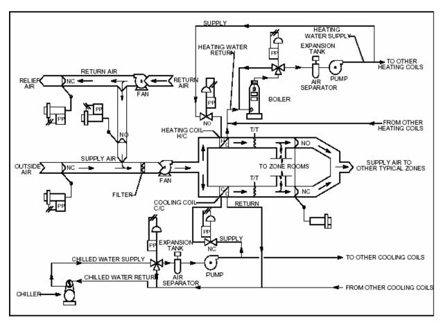
Figure 4-1. Schematic of a typical HVAC system
