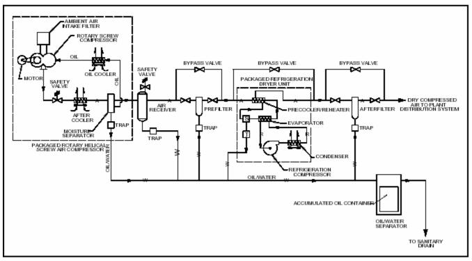
Figure 6-1 Schematic of a typical compressed air system
