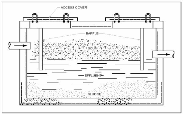
Figure 9-3 Cross Section of a Septic Tank
