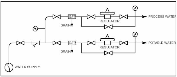
Figure 9-1 Schematic of a Typical Potable and Process Water System
