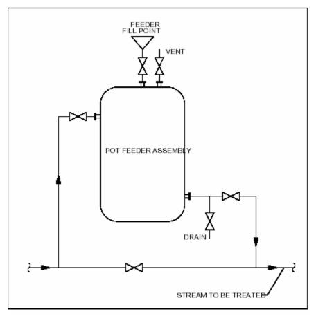
Figure 9-2 Schematic of a Process Water Treatment System
