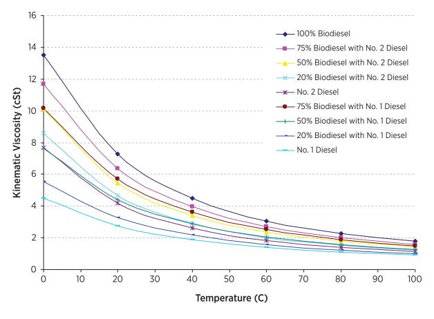
Figure 16. Kinematic viscosity for a commercial biodiesel in various blends<sup>30</sup>
