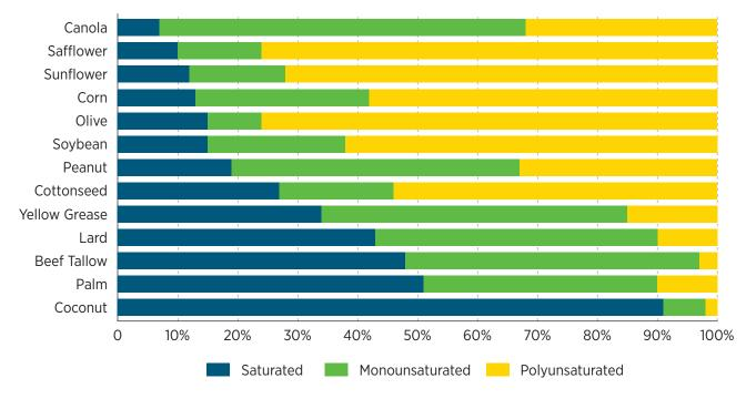
Figure 2. Composition of various biodiesel feedstocks in order of increasing saturated fatty acid content
