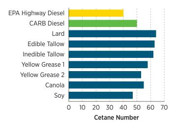
Figure 3. Cetane numbers of two petroleum diesels and several biodiesels
