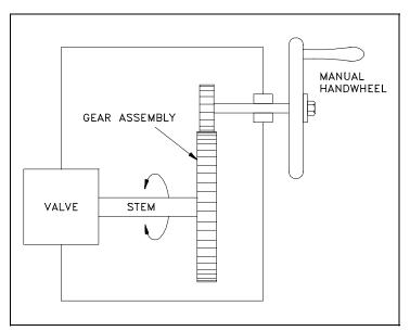
Figure 32 Manual Gear Head
