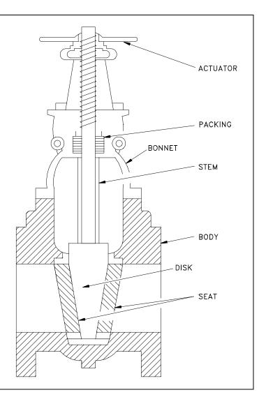
Figure 1 Basic Parts of a Valve
