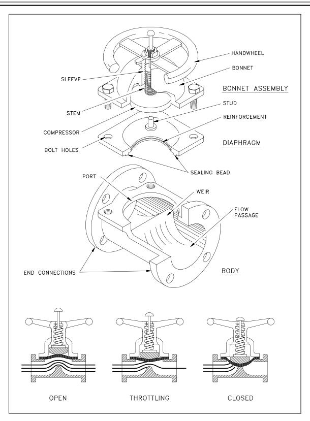
Figure 15 Weir Diaphragm Valve
