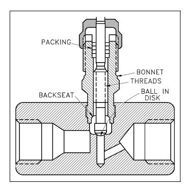
Figure 21 Bar-Stock Instrument Valve
