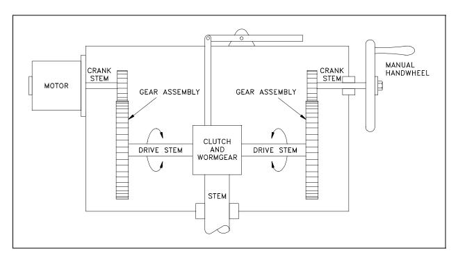
Figure 33 Electric Motor Actuator
