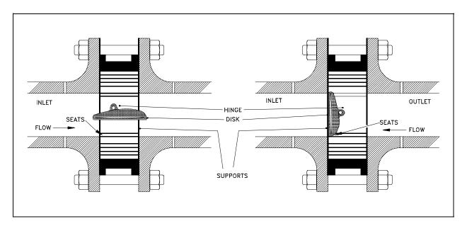
Figure 23 Operation of Tilting Disk Check Valve
