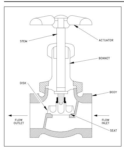
Figure 27 Stop Check Valve
