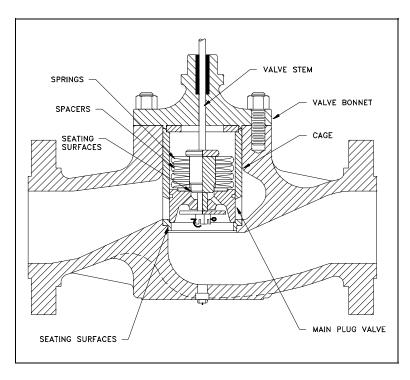
Figure 25 Piston Check Valve
