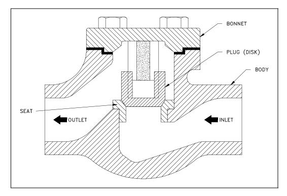
Figure 24 Lift Check Valve
