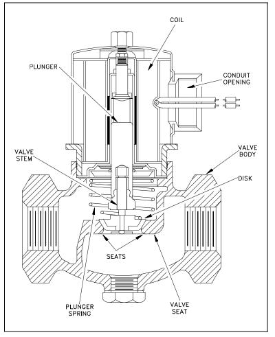
Figure 35 Solenoid Actuated Valve
