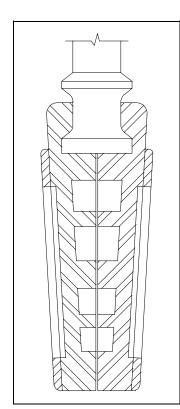
Figure 6 Flexible Wedge Gate Valve
