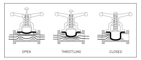
Figure 14 Straight Through Diaphragm Valve
