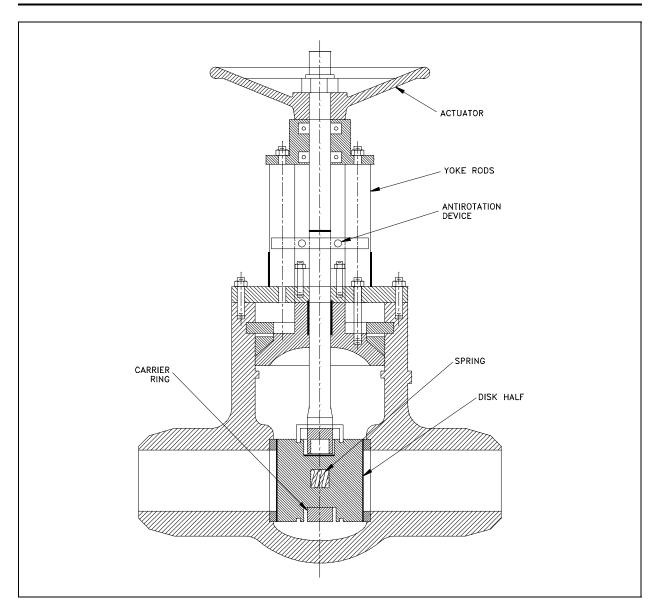
Figure 8 Parallel Disk Gate Valve
