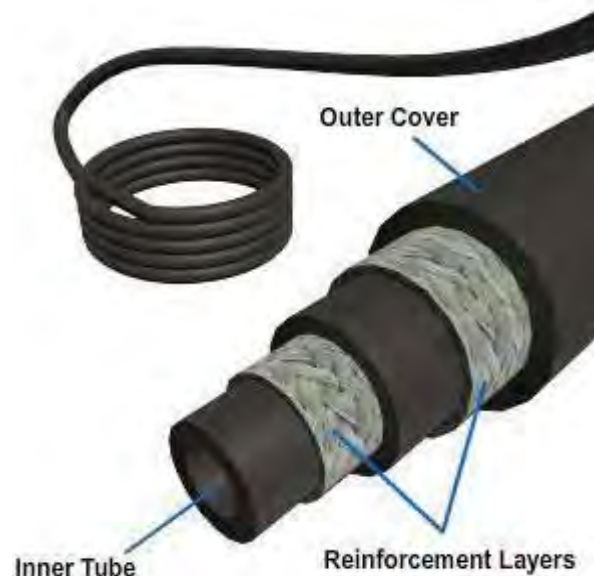
Figure 25 — Flexible rubber hose construction.
