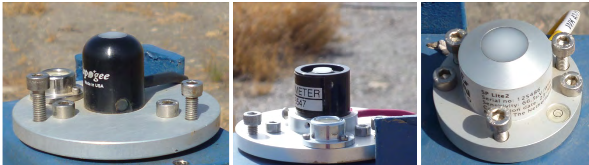
Figure 2-10. Selected photodiode sensors with different diffusor geometries. Photos by DLR
