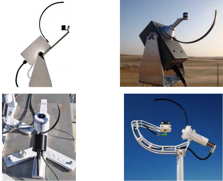
Figure 2-15. Four commercially available RSIs (clockwise from top left): Irradiance, Inc., model RSR2; Reichert GmbH RSP 4G; Yankee Environmental Systems, Inc., model SDR-1; and CSP-Services GmbH Twin-RSI. Photos by (clockwise from top left) Irradiance, Inc.; CSP-Services; NREL; and CSP-Services
