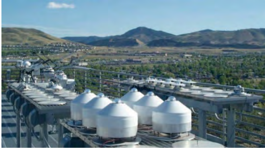
Figure 2-9. Kipp & Zonen model CM22 pyranometers installed in ventilated CV2 enclosures. Photo by NREL
