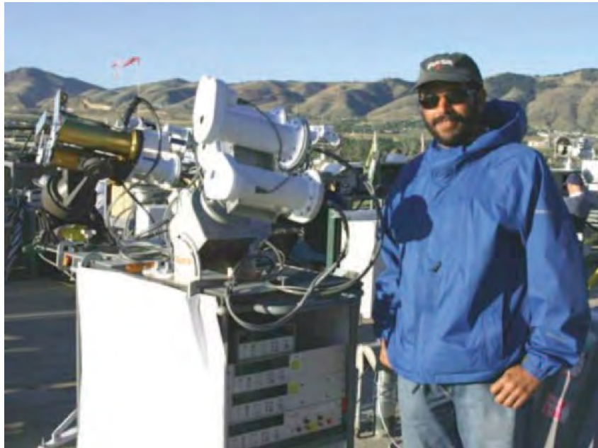
Figure 2-5. Multiple electrically self-calibrating absolute cavity radiometers mounted on solar trackers with control and data acquisition electronics. Photo by NREL
