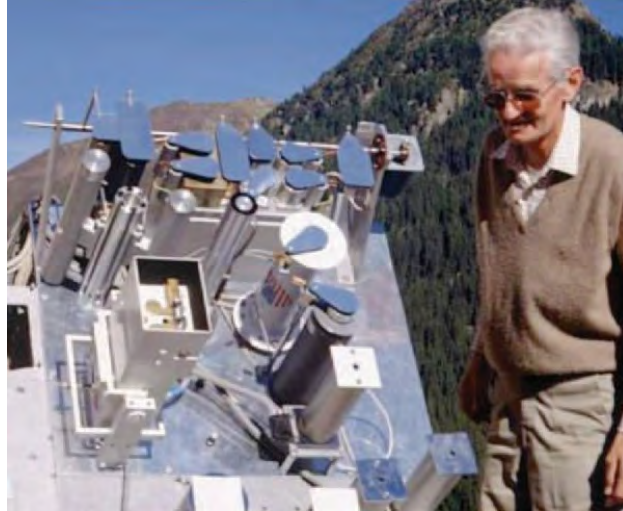
Figure 2-6. The World Standard Group of six absolute cavity radiometers is used to define the WRR or DNI measurement standard. Photo by NREL
