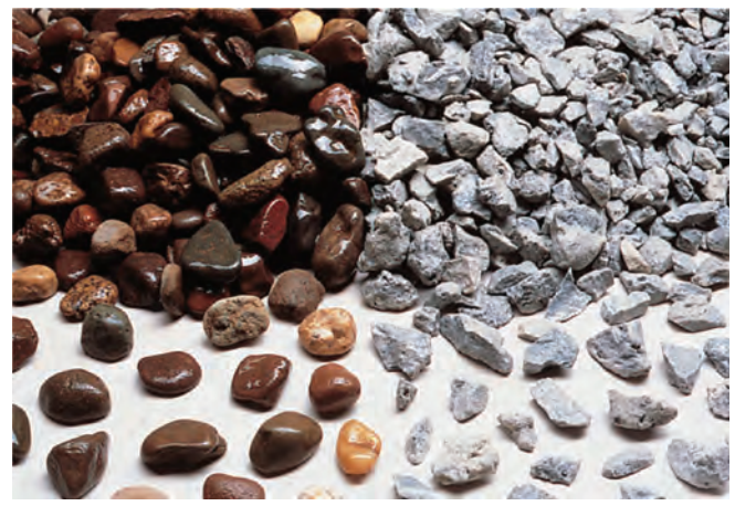
Figure 4.7 Rounded (left) and crushed natural aggregates (photo courtesy of Portland Cement Association)
