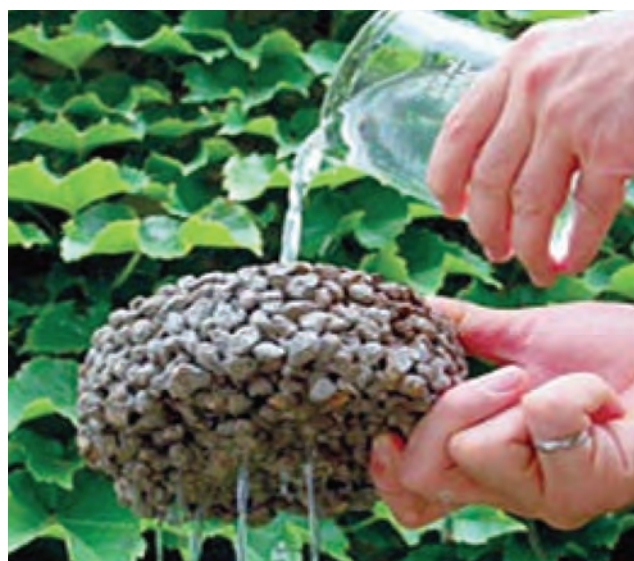
Figure 9.3 Water passing through pervious concrete (NRMCA 2009)
